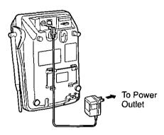
Tuck the telephone line cord inside the wall mounting adaptor, then push it in the direction of the arrow.
